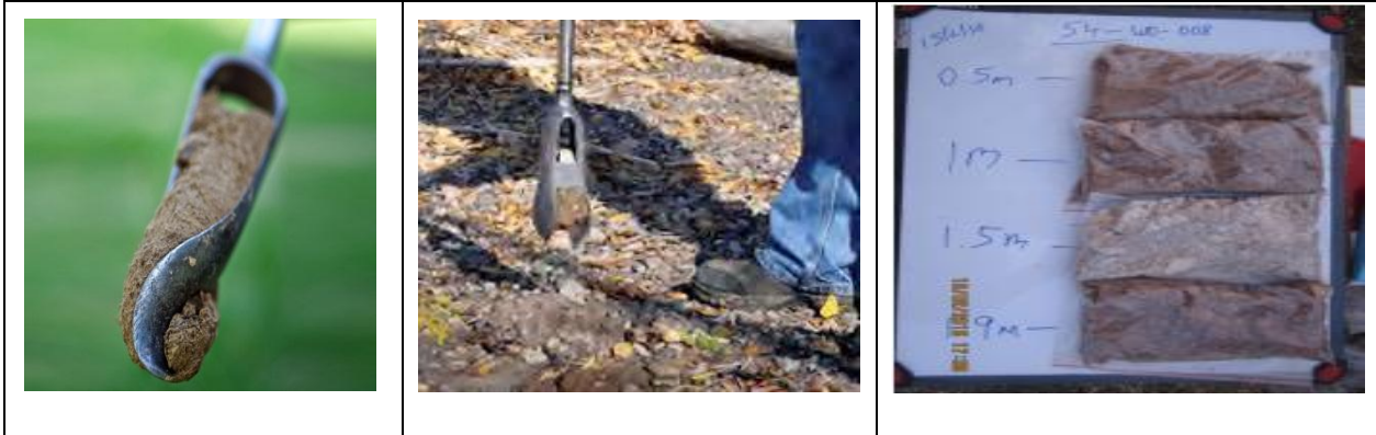
Examples of soil sampling with Edelman auger
