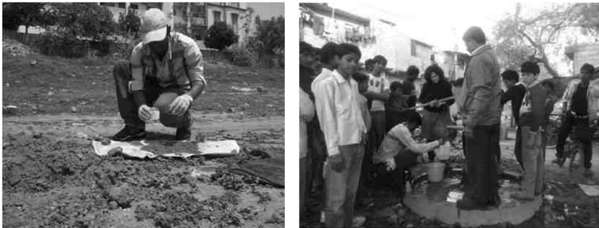
Figure I-2.1.1a and 1b: Sampling of soil and groundwater (pictures by COWI, Kadam)
