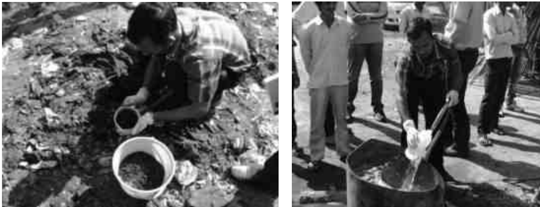
Figure I-2.2.2a and 2b: Sampling of soil and groundwater (pictures by COWI, Kadam)
