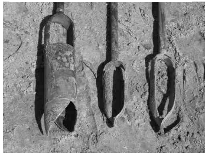
Figure III-2.2-ii.5b Example of augers. From left to right: Riverside (gravel, debris), auger (sand), Edelman auger
