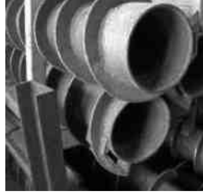
Figure III-2.2-ii 4. Hollow auger drill
