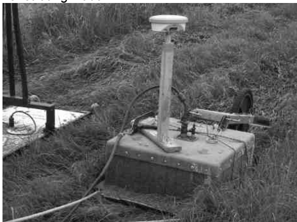
Figure III-2.2-ii.1a and 1b: Example of Ground Penetrating Radar
