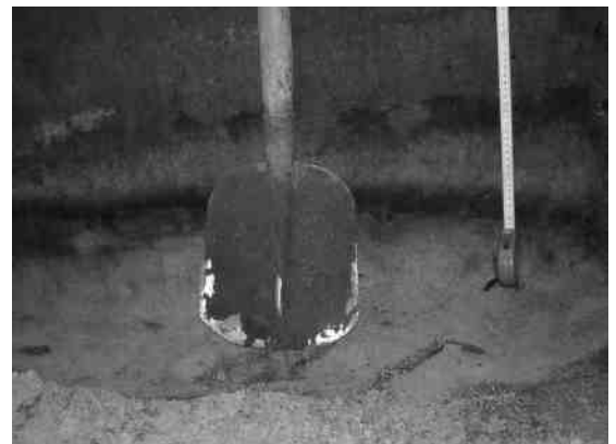
Figure III-2.2-ii.4b Example of trial pit excavated with shovel
