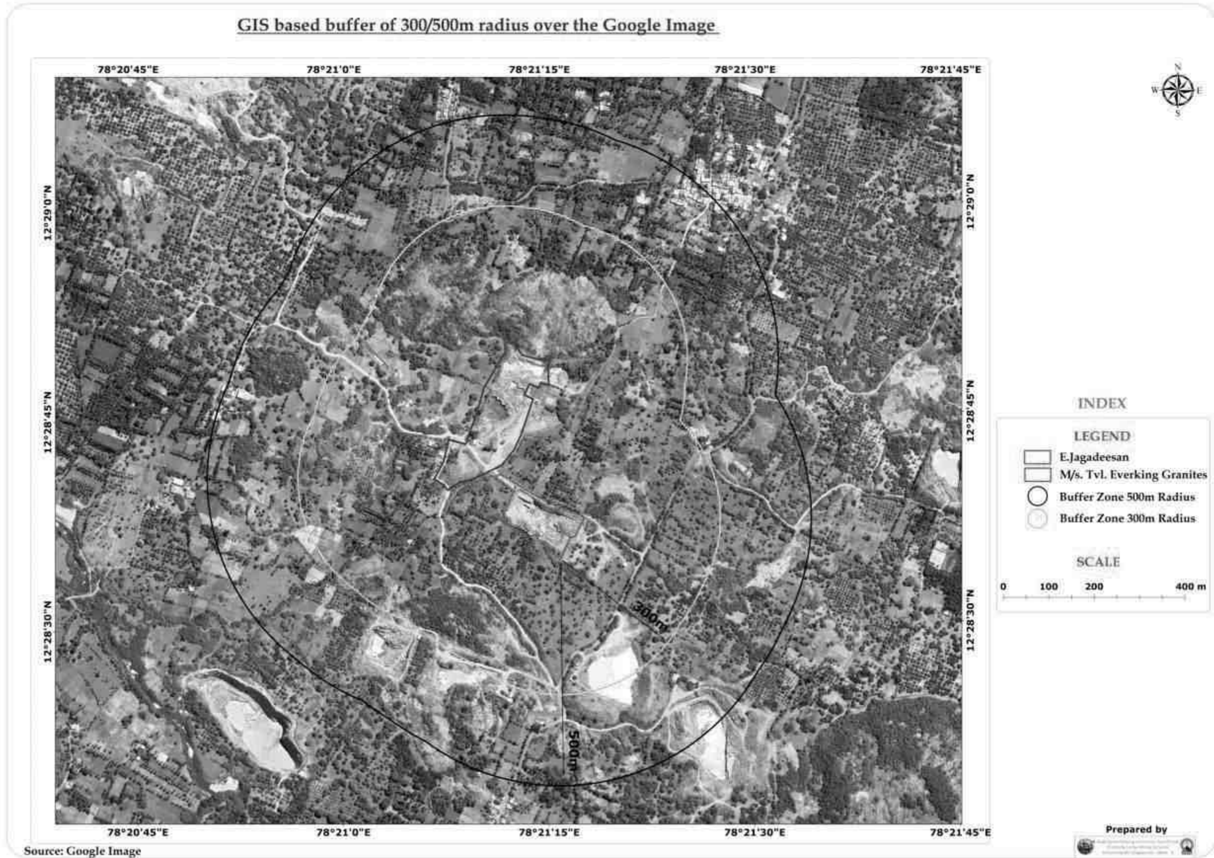
Fig 1.3: Google Earth Image showing 300m and 500m radius around two existing grey granite quarries
