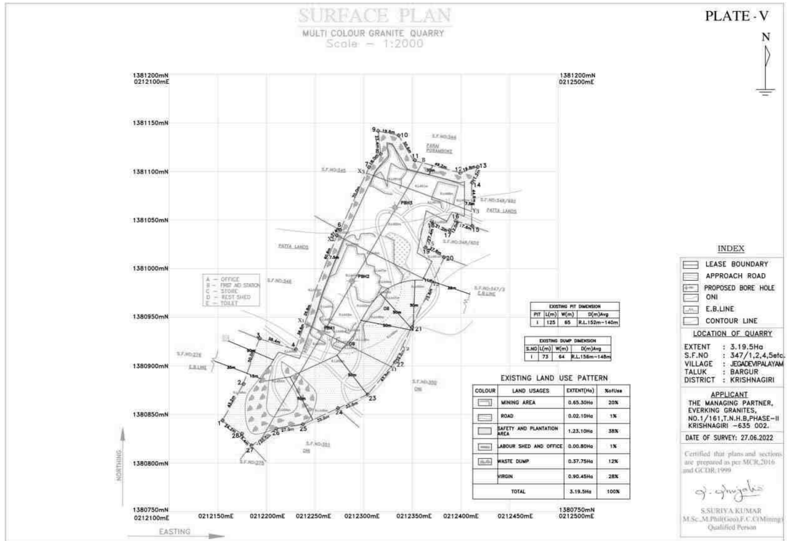
Fig.No.2.3: Surface Plan of Existing Grey Granite Quarry of Tvl. Everking Granites (3.19.5 Ha)
