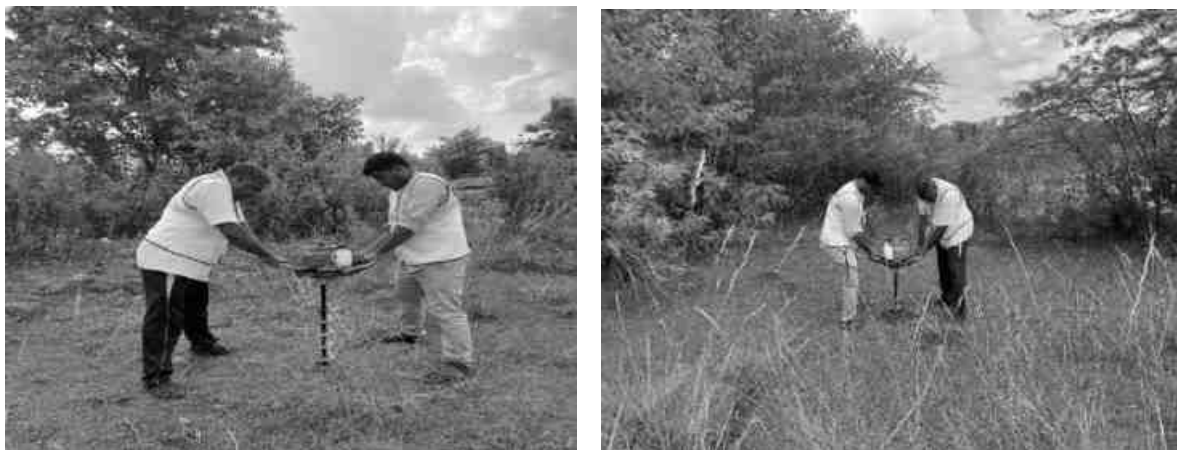
Figure 3.20 Soil Sample Collection using Motorized Auger for Soil Chemistry Analysis.
