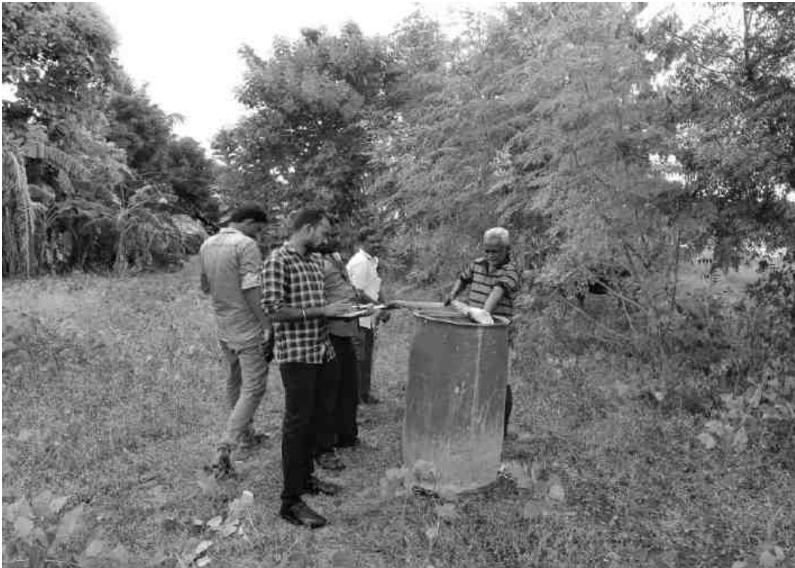
Fig No: 3.13 Photograph showing measured by discharge water (LPM) in well
