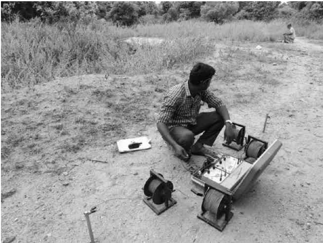
Fig No: 3.12 Photos showing Electrical Resistivity survey conducted at near Palar River in Kuthambakkam village
