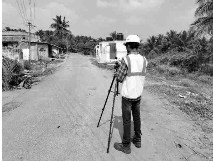
FIGURE 3.15: SITE PHOTOGRAPHS OF AMBIENT NOISE LEVEL MONITORING
