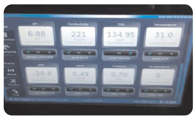
Online water quality monitoring system installed in River Cauvery
