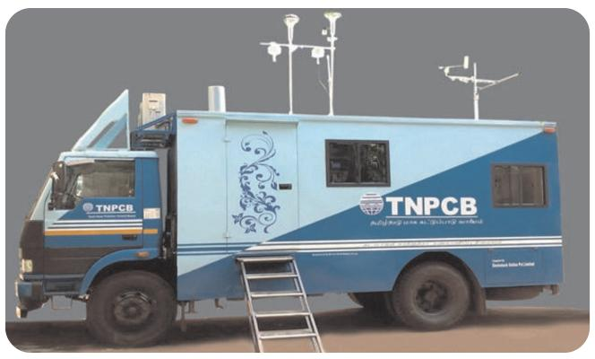
MOBILE CONTINUOUS AMBIENT AIR QUALITY MONITORING STATION (Mobile CAAQMS)
