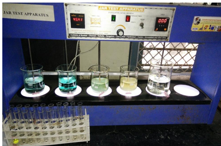
Fig. 1: Reduction of hexavalent chromium using sodium metabisulphite
