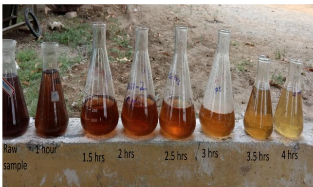
Fig.1 - Ozone treatment of tannery effluent
