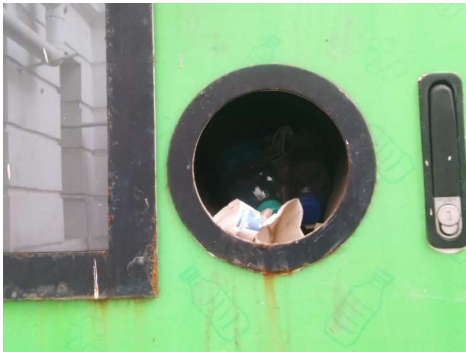
Figure 24: Clogged Reverse Vending Machine placed next to the Tamil Nadu Urban Rural Mission tea stall
