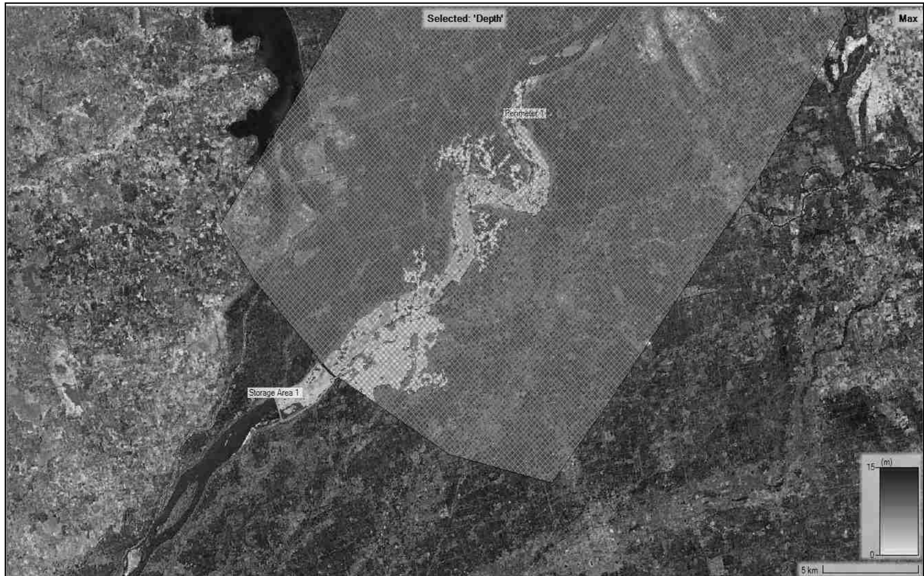
Fig Map 7.3 Image of Dam break analysis showing depth of flood water in the inundation area (Bing Satellite Map)
