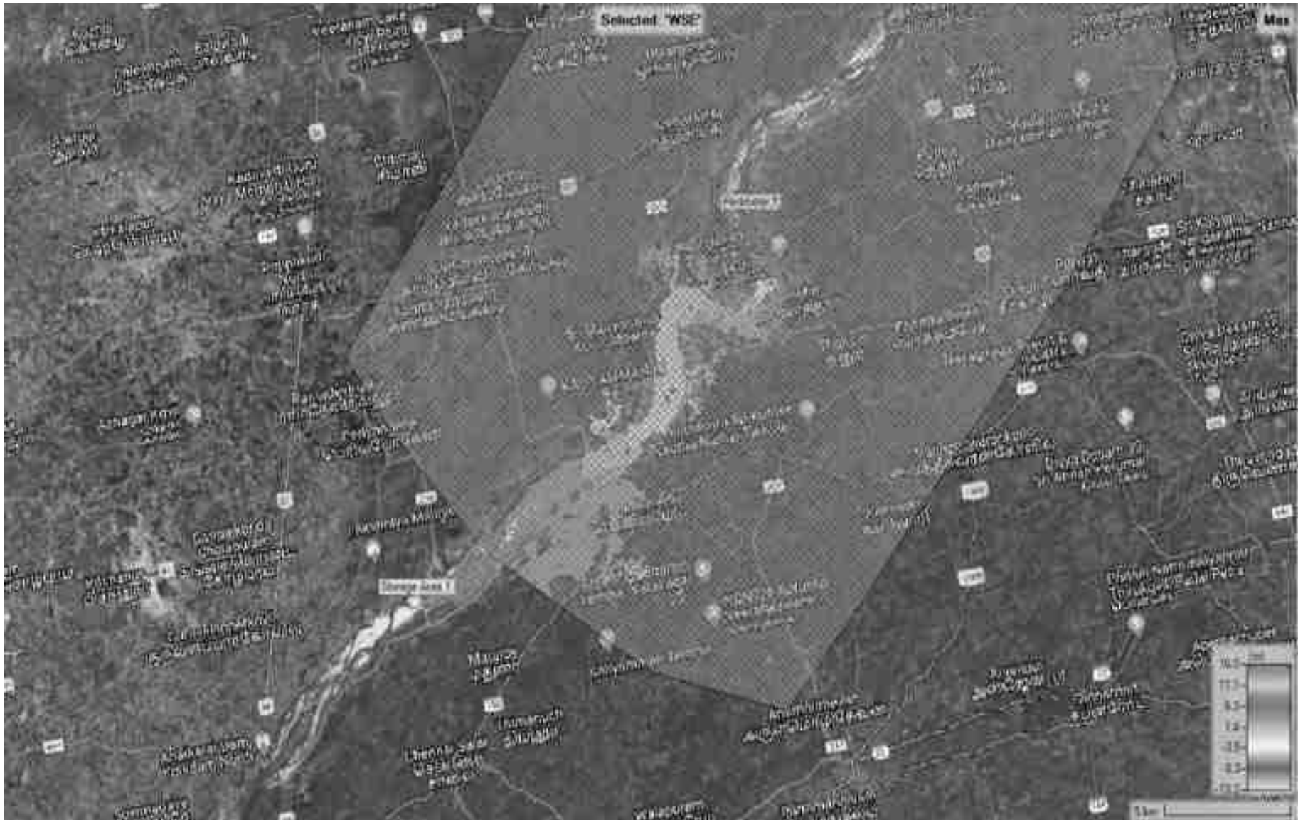
Fig Map 7.5 Image of dam break analysis showing elevation of water surface level over inundation area (Satellite Map)
