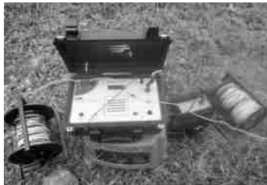
Figure 4. Electrical resistivity survey Instruments.
