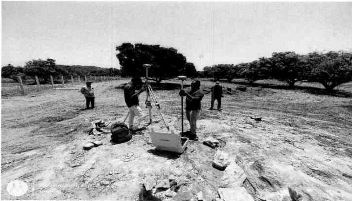
Fig.1 Photographs showing DGPS Survey of the base point
