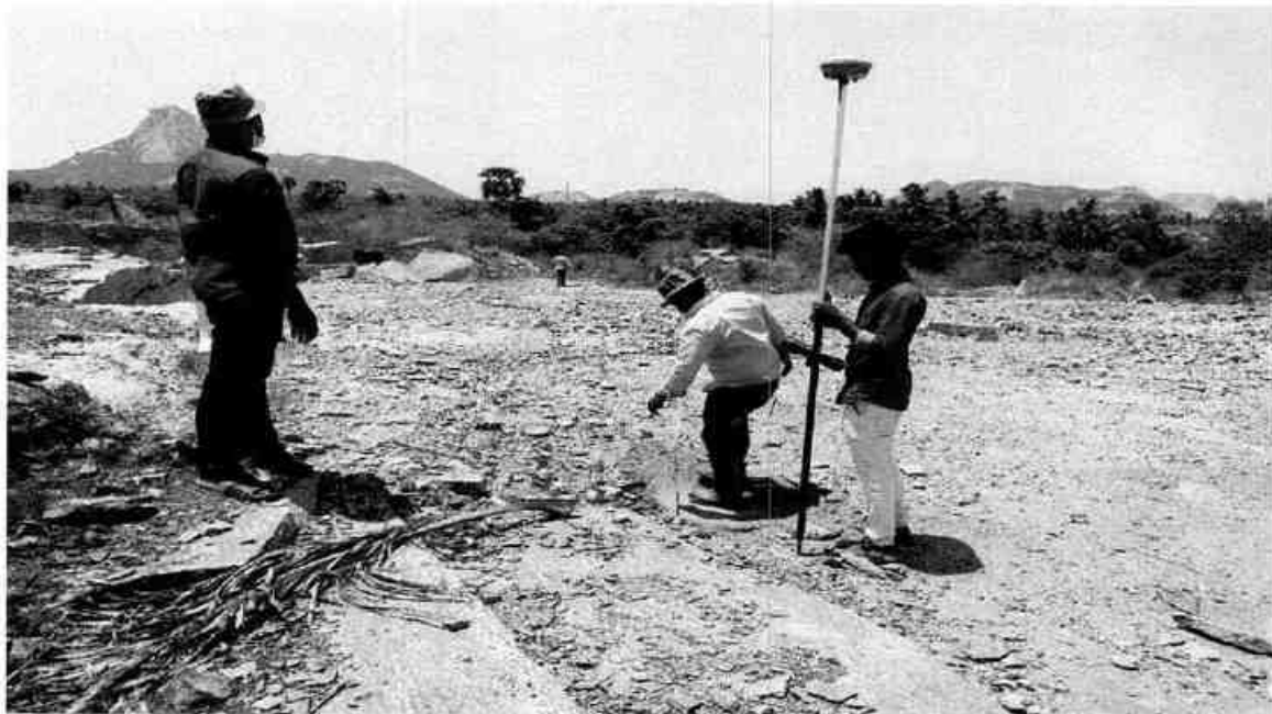
Fig.2 Photographs showing DGPS Survey of the rover unit
