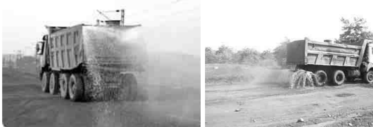
FIGURE 10.1: WATER SPRINKLING ON HAUL ROADS
